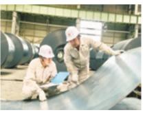
Checking the quality of steel plate surface
