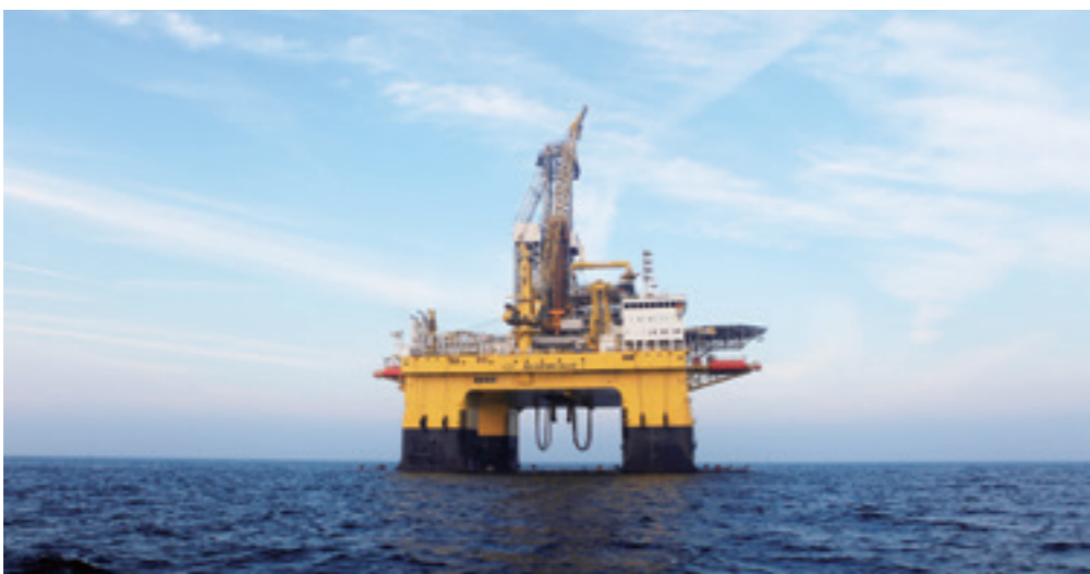
Blue Whale I using the TMCP form Grade F super strength marine steel of Ansteel
