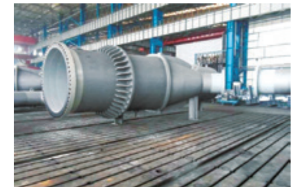
Ansteel steel plate ADB610D used for hydropower in Ecuador
