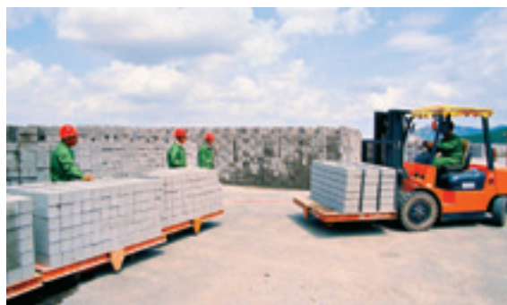
Air Bricks Made from Tailings
