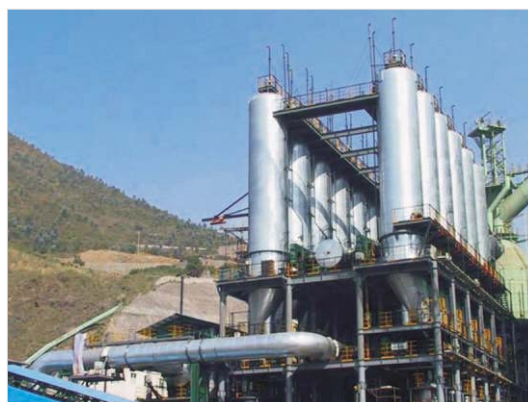
▲ Power generation device by the waste pressure from the new No. 3 blast furnace of Panzhihua Steel & Vanadium Co., Ltd.
