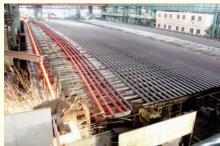
is rolling high-speed steel rails.
